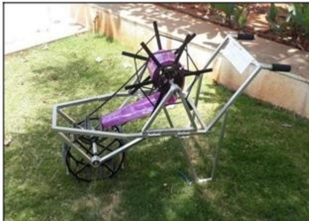
*Fig.5 Actual model with reeled pipe*
